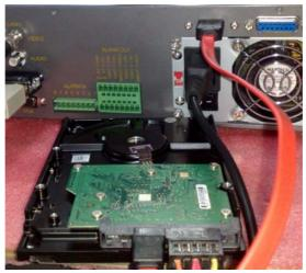
Fig. B-2 Normal Hard Drive Connection
